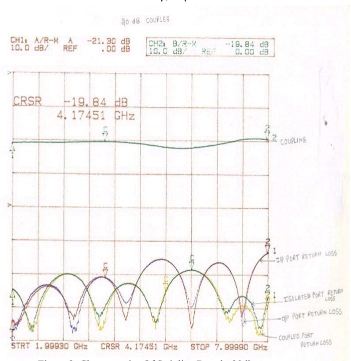
Figure 2: Characteristics Of Stripline Based -20db Coupler From Network Analyzer.
