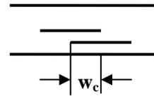
Figure1. Overlap Coupled parallel lines
