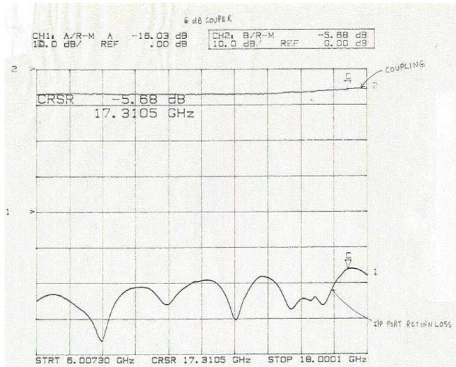
Figure 3. Plot of coupling and input port return loss of a 6db coupler
